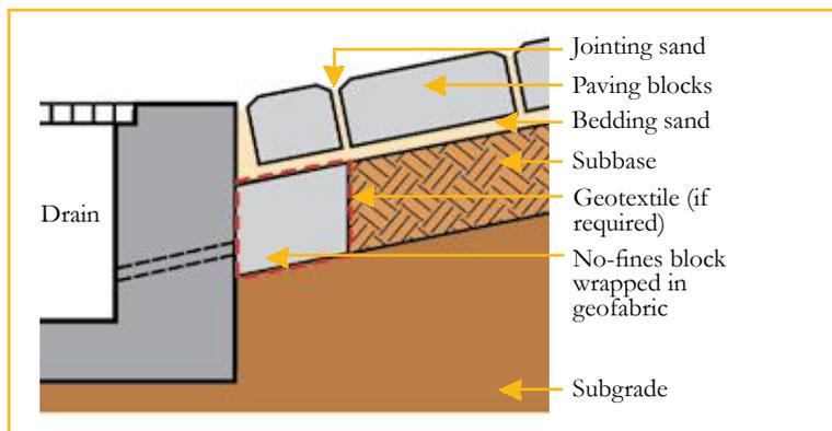
**Figure 3 a** – No fines block in subbase layer
