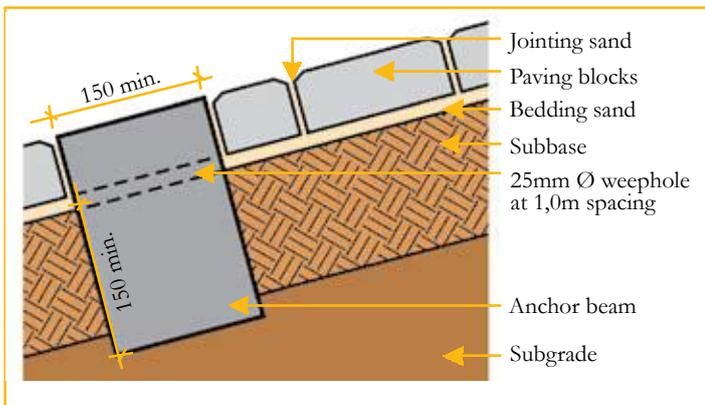
**Figure 1** – Typical section through anchor beam showing dimensions
