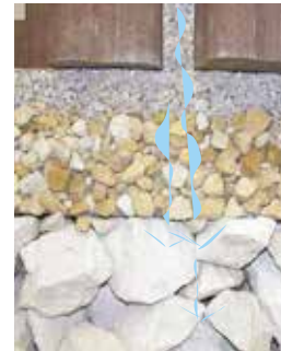
Permeable interlocking concrete pavement (PICP) with open-graded base and subbase for infiltration and storage.
